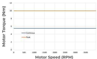
EHPU-1-56-XXX-U-SAE Frame Size 1 56 mm motor 350-800Vdc
