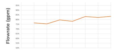
Pump Speed (rpm)
