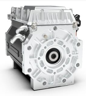
The Terzo Power, Frame Size 3, Electro-Hydraulic Power unit is the only motor on the market specifically designed around the needs of hydraulic systems in the EV market, focusing on ease of integration and efficiency. The standard SAE B Mounting interface, builtin pressure sensors, and pressure control modes allow for true plug and play integration and Power on Demand control.
